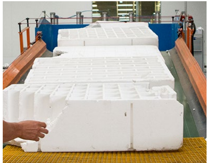
EPS offcuts being recycled at Unipod®.
